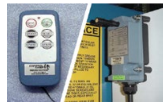
WIRELESS REMOTE: Receiver mounts to machine
