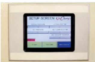
HMI OPERATOR INTERFACE: Offers multiple screens for maintenance and pressure settings
