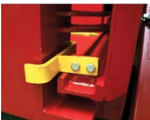
LOCK OUT BAR: Prevents plates from moving when maintenance is required
