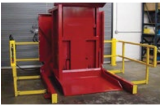
STANDARD MACHINE GUARDING: Provides protection from forklifts
