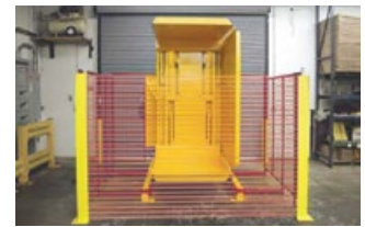
LIGHT CURTAINS: Provides a soft guarding across the front of the machine for additional protection
