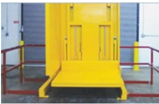
STANDARD MACHINE GUARDING: Provides protection from forklifts
