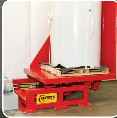
Rotate product within a 90-degree radius to change vertical/horizontal orientation for shipping or production.
