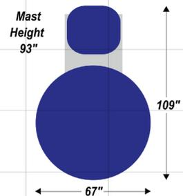
\* Maximum wrap height may vary based on film force, neckdown, and roll carriage travel speed.
