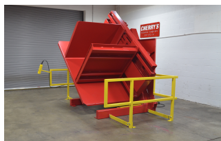
STANDARD MACHINE GUARDING: Provides protection from forklifts
