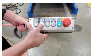
PUSH BUTTON: Comes on a 30-foot cord with E-stop, lock out tag/out and pendant holder
