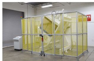
BOSCH GUARDING: Guarding which bolts directly to the floor with removable panels for maintenance access
