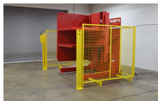
HIGH STYLE GUARDING: Provides additional protection for forklift operators (mounted directly to the machine)
